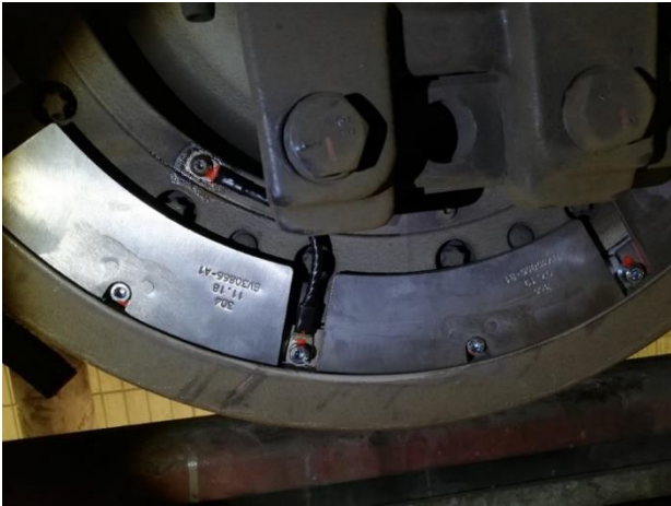
Figure 3: Shunts and absorbers installed on the aluminium hybrid wheel [3]
